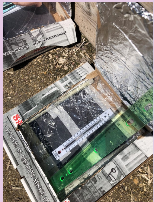
Picture of what the set up solar oven looked like. Each oven was propped open with a ruler and had a thermometer inside.
